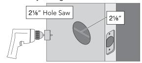
3c If necessary, enlarge hole in door edge.
