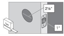
3b If necessary, enlarge hole in door face.
