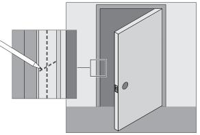
6b Measure, mark and drill two (2) 1" holes, 1 ¼" deep, as shown. Chisel out excess material on the sides.
