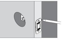
5b Remove bolt and drill two <sup>1</sup>/<sub>8</sub>" pilot holes.
