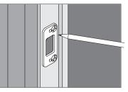
4c If necessary, use chisel, hammer and drill to correct door jamb preparation.
