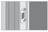
4b If correction is necessary, trace faceplate and mark holes.
