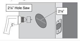
3c If necessary, enlarge hole in door edge.
